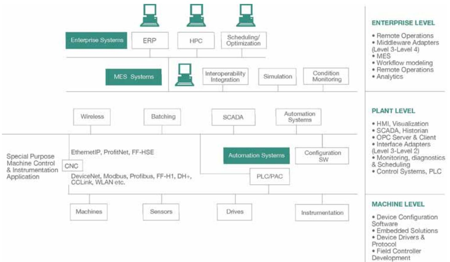
**CNC** – Computer Numerical Control, **CCLink** – Control and Communication Link, **ERP** – Enterprise Resource Planning, **HMI** – Human Machine Interface, **HPC** – High Performance Computing, **MES** – Manufacturing Execution System, **OPC** – Object Linking and Embedding (OLE) for process control, **PLC/PAC** – Programmable logic Controllers / Programmable Automation Controller, **SCADA** – Supervisory Control and Data Acquisition, **WLAN** – Wireless Local Area Network
