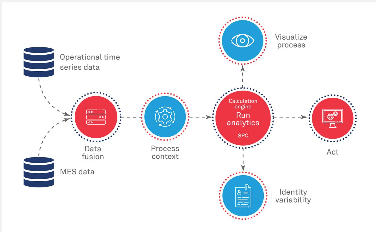
Process Monitor uses SPC charts, powerful calculating functions and models that allow users to visualize variability in process from one production run to the next. This allows operations to immediately investigate the root causes of variability, machine breakdowns, waste, etc., and then act to drive consistency and improvement across runs (see above how ProcessMonitor works).
