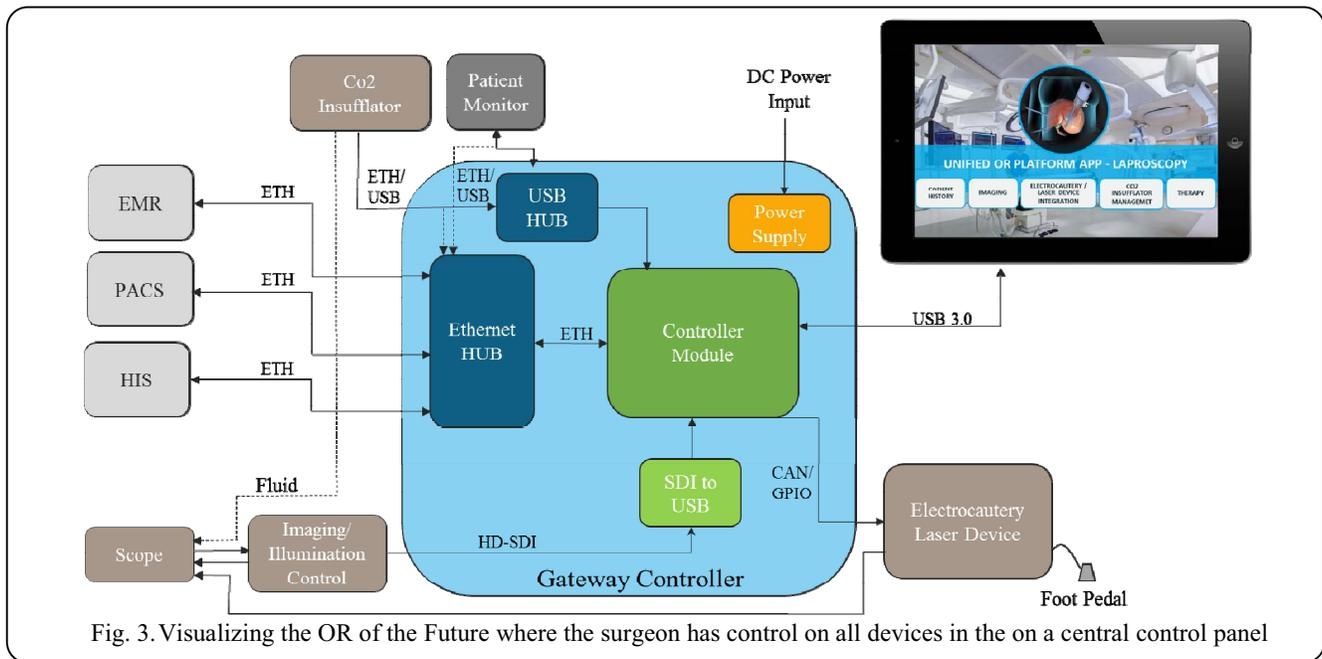
Fig. 3. Visualizing the OR of the Future where the surgeon has control on all devices in the on a central control panel
