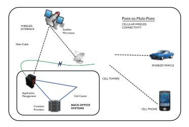
Data is either generated in the vehicle unit and gets relayed to the back office systems or the back office systems push data like maps, weather forecasts, stock updates, Internet data packets etc to the vehicle unit. This communication takes place either through the cell phone or the unit fitted in the vehicle itself. The communication and location mapping for the vehicle happens through a network of cellular towers and satellite systems.
