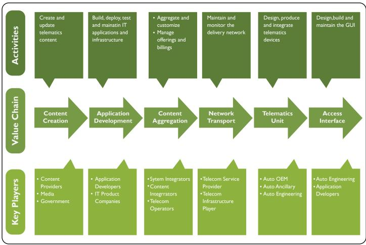
The core value in the telematics value chain is the data content. The source of the data content is either the vehicle's systems that track parameters related to the vehicles performance or external/ third party media content beamed in through the telecommunication networks. From left to right, data flows from the source to the target.
