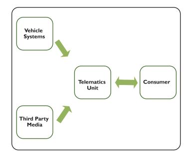
Telematics Unit is the communication component that talks directly with the vehicle. There are two data sources for the unit – the vehicle itself and third party media content beamed from the outside world. This third party content is primarily Internet driven data, voice and video content provided by web portals. The consumer can either be the vehicle driver/ passengers accessing the data or the entities that want to use vehicle generated content.
