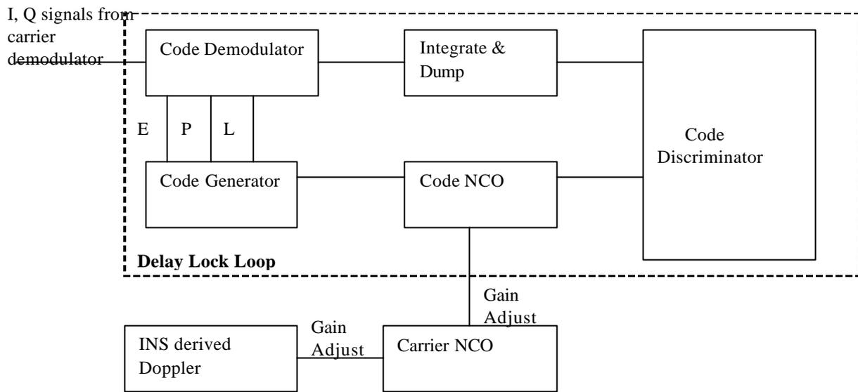
**Figure 2. Ultra-tight Code Tracking Loop**
