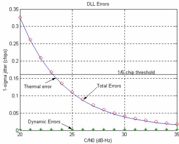
Figure 5. DLL Errors (Thermal, Dynamic and Total)
